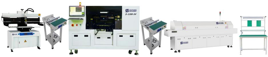
Semi-Auto Screen Printer → Buffer Conveyor → Pick and Place → Buffer Conveyor → Reflow Oven → Worktable
